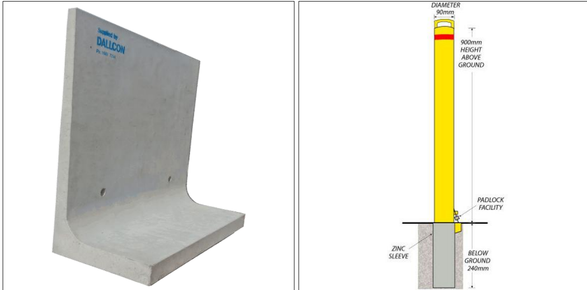
Figure 5.5 - L-block and Safety Bollard
