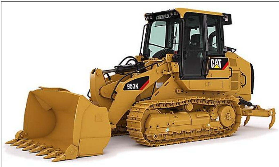
Figure 5.6 - Cat 953K Tracked Loader
